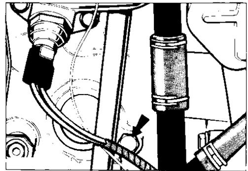
Cylinder block drain bung.
