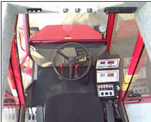
Operator's view showing fingertip controls
