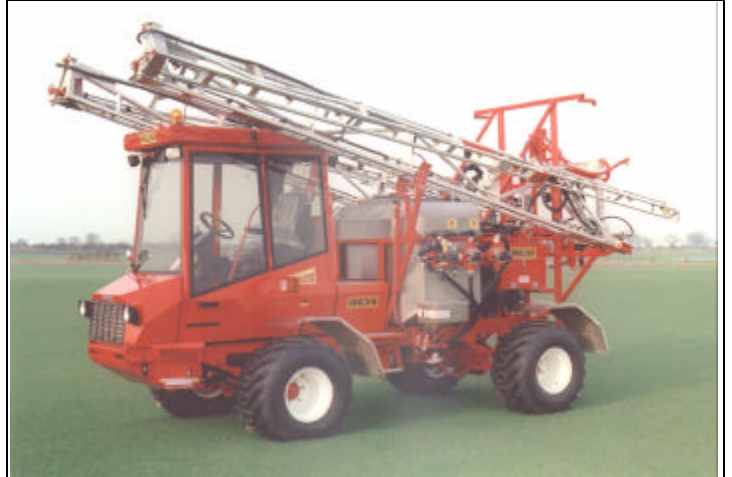
The Phantom with 1600litre, 24m lightweight sprayer
